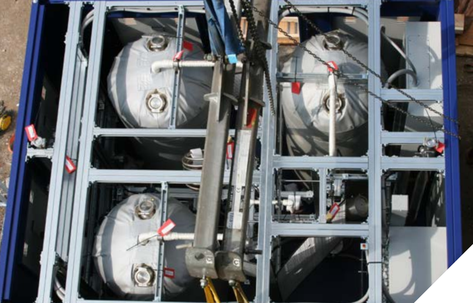
Large purifiers system ready to be lifted into the building.
