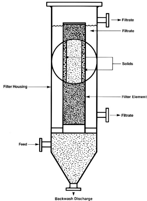
**FIGURE 2: Design Schematic of HyPulse LSI Filter**
