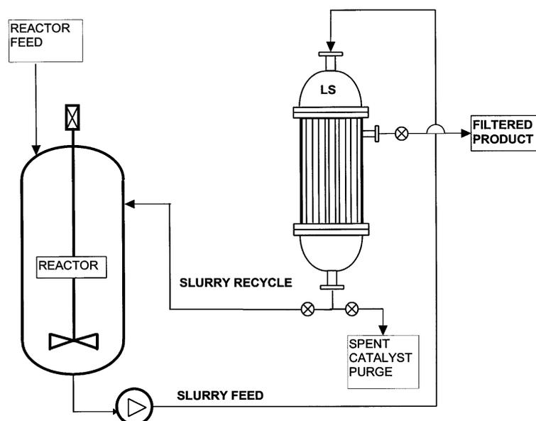
The HyPulse LSM filter utilizes double open-ended porous metal filter elements (see
