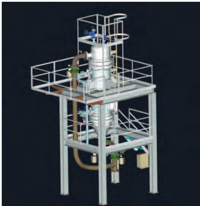
Skid-mounted Mott HyPulse LSM system used for catalyst recovery.
