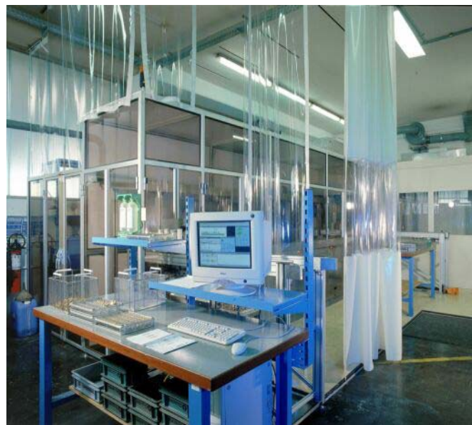
Cleaning station SERTO AG
