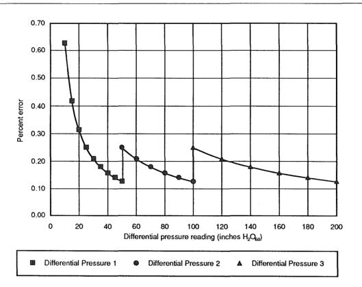
Note: The precision of the differential pressure device used in this example is ±0.25 percent of full scale.
