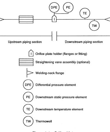
Figure 1-1—Orifice Meter
