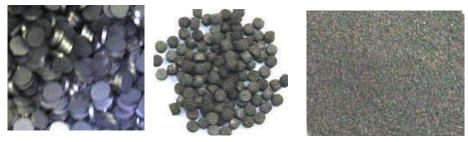
Typically Removes: CO, CO<sub>2</sub>, H<sub>2</sub>, H<sub>2</sub>O, N<sub>2</sub>, O<sub>2</sub>, THC
